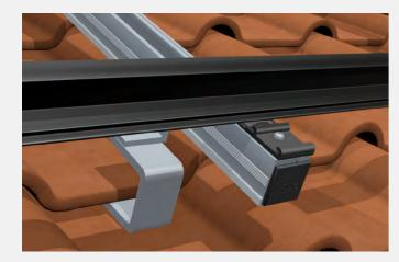
3. Clicking the TS insert profiles into the SafeClick The insertion profiles are clicked into the SafeClick and are floatingly connected to the roof. Damage to the roof and module caused by thermal expansion is thus avoided.
