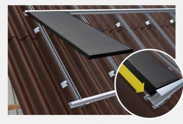
**4.** Inserting the modules into the TS insertion profiles The modules are inserted into the insertion profiles and are held in place by their own weight - there is no need for additional fastening.
