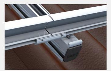
3. Clicking the TS insert profiles into the SafeClick The insertion profiles are clicked into the SafeClick and are floatingly connected to the roof. Damage to the roof and module caused by thermal expansion is thus avoided.
