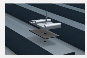
2. Riveting the SafeClick onto the trapezoidal sheet The proven SafeClick is mounted directly onto the trapezoidal sheet metal by rivet1, whereby considerably fewer fastening points become necessary.
